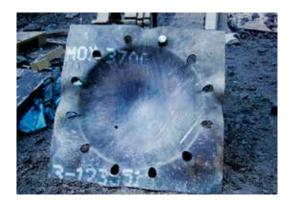
ARMOX 370T has the highest toughness in our range. Its superior toughness makes this steel a common choice for applications with high requirments on blast protection. The purity and composition of the steel also makes the steel easy to process, including excellent properites for welding and bending.
